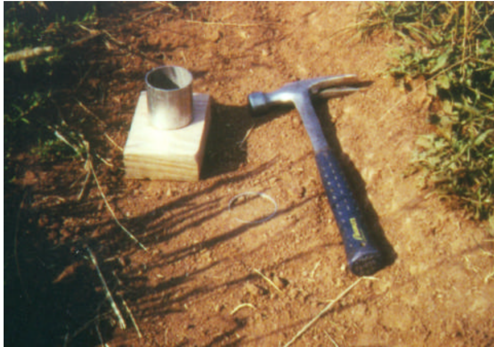
Figure 8: Core sampler in center of trail.
