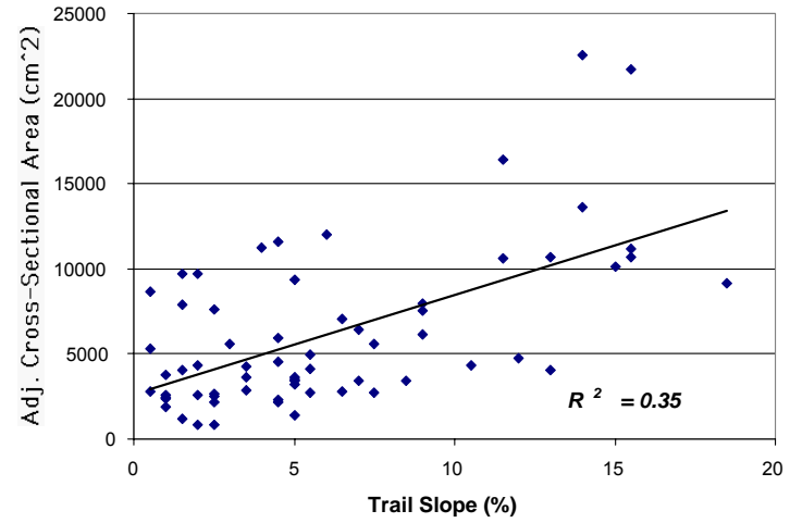
Figure 13: Measured and adjusted cross-sections vs. trail slope.
